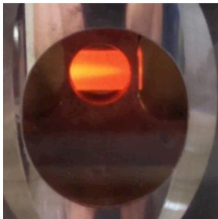
Figure 2.6: *Fluorescence from 527.5 nm Excitation.* Fluorescence from shining 527.5 nm laser through the crystal while it is cooled to liquid helium temperatures. In this picture the green laser is traveling from left to right. As the beam gets further into the crystal the profile tapers off as a result of absorption.
