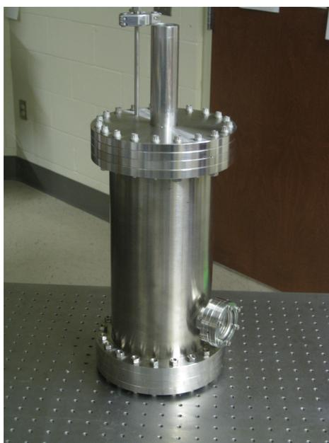
Figure 2.1: *Liquid Nitrogen Chamber*. This chamber was used to cool the crystal to liquid nitrogen temperatures and to do the initial spectroscopic measurements on our YSO crystal. A roughing pump was hooked up to the thin pipe with the KF flange and liquid nitrogen was poured into the larger diameter pipe on the top. The viewport provided optical axis to the crystal.
