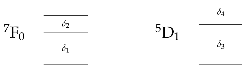
Figure 4.6: The levels on the left are the {}^7F_0 hyperfine states with splitting \delta_1 and \delta_2 . The levels on the right are the {}^5D_1 hyperfine states with splitting \delta_3 and \delta_4 . All values are in MHz.
